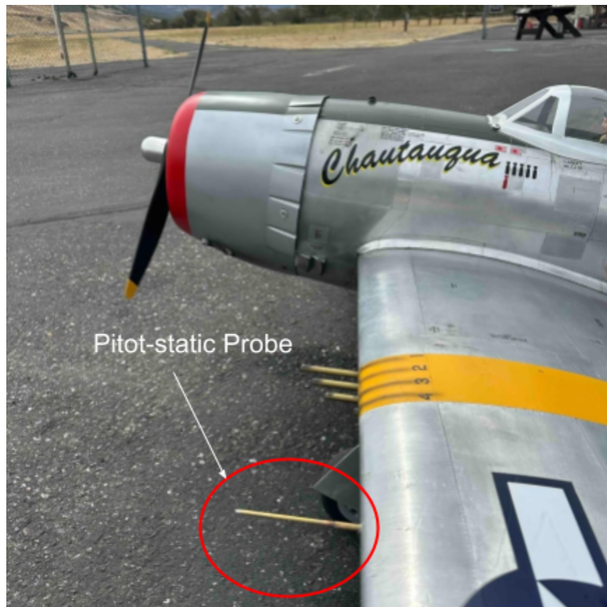
Giant Scale P-47 Warbird with a custom made probe.
