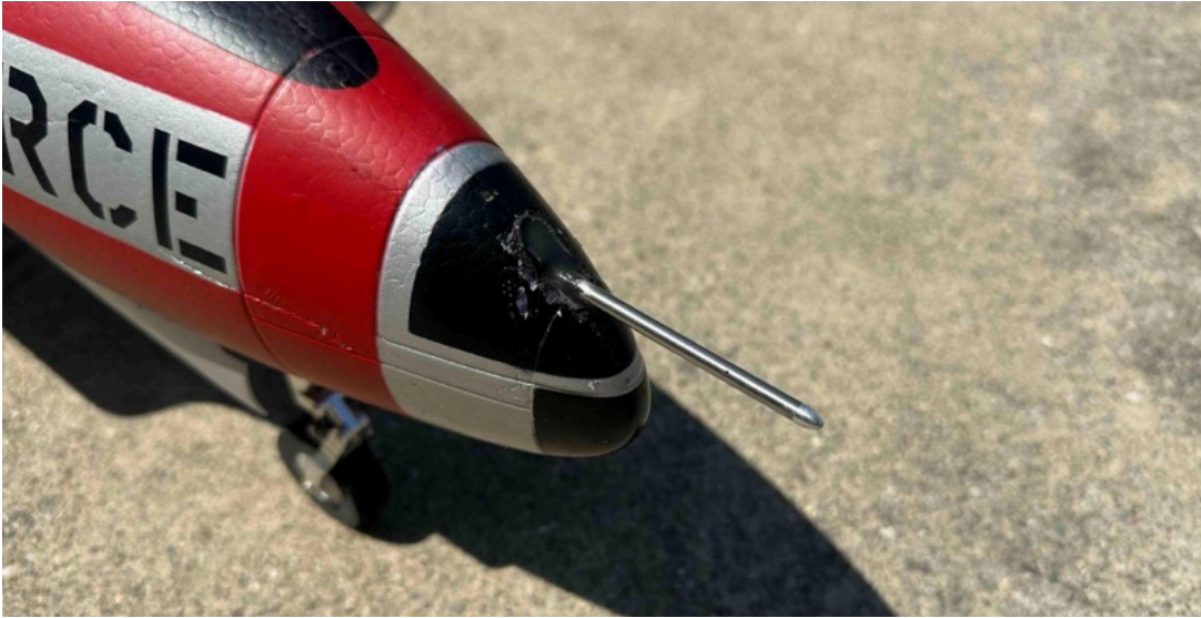
Nose of T-33 EDF with pitot-static probe using an off the shelf-probe available from RCATS.
